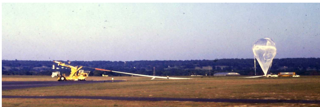
Fig 13: Just before launch. The partially filled balloon fills out at high altitude. The balloon is released at the right side and the launch vehicle "Tiny Tim" manoeuvres downwind beneath it, holding the payload until the balloon takes the load.
