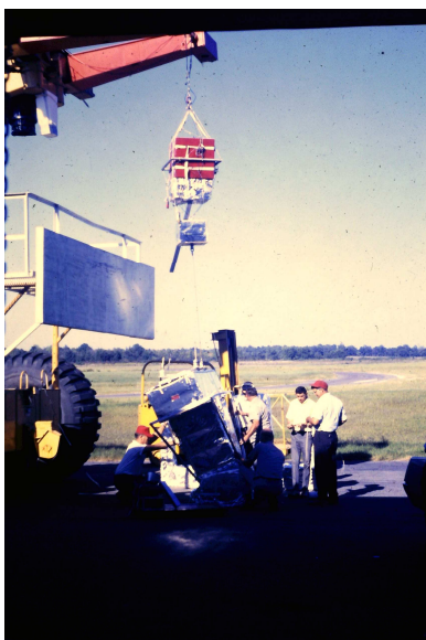
Fig 12: The gondola is covered with insulation and reflective foil. It is suspended from a line twister and above it is the chute for lead shot from the red
