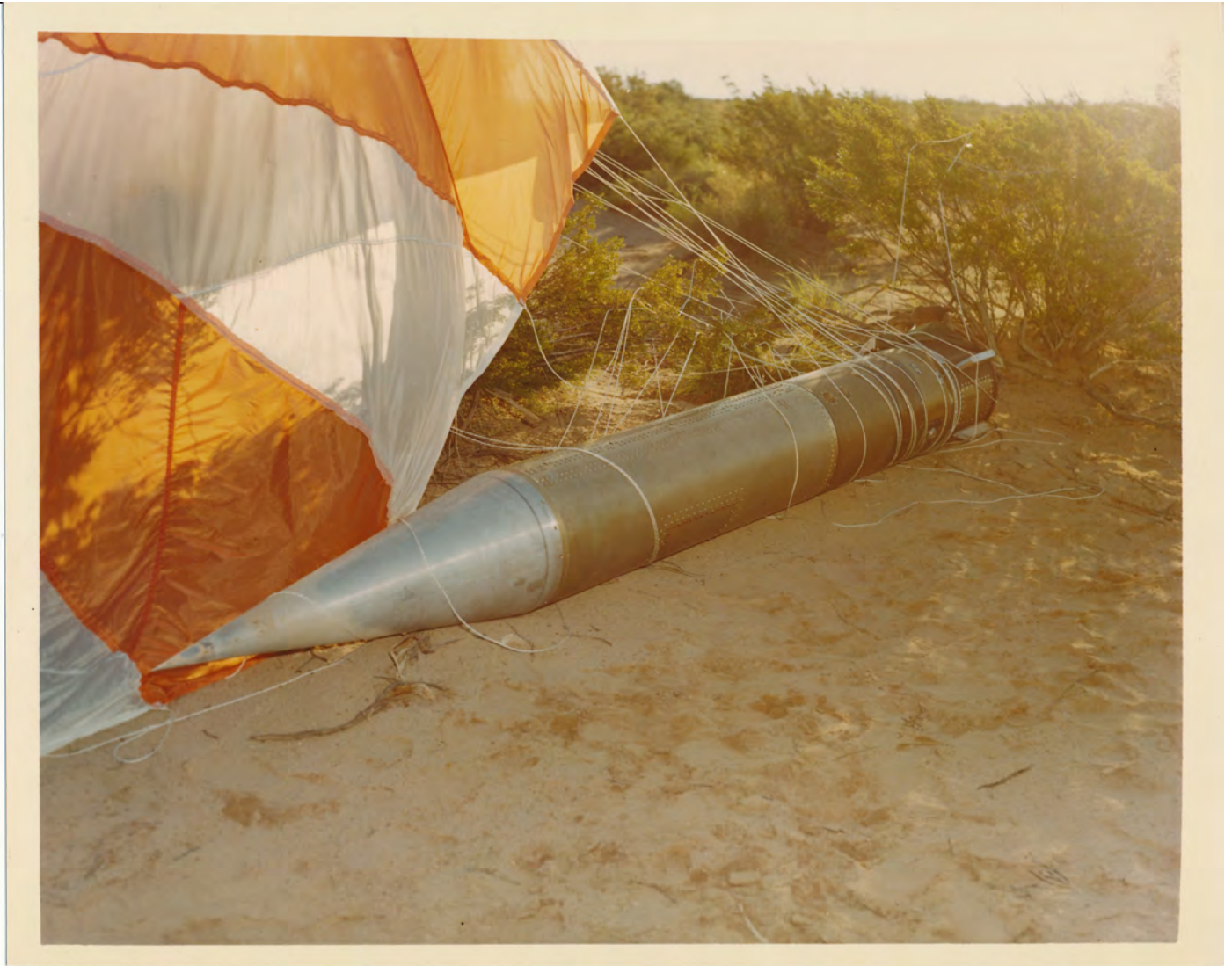
Recovery of NASA/MIT Rocket payload 4.225, 26 July 1968. The parachute is deployed from the lower (right) casing when the falling and tumbling payload reaches about 20,000 feet altitude. The payload includes the MIT experiment and also guidance and telemetry packages provided by GSFC. GSFC provided the experiment payload cylinder and door. (NASA Photo)
